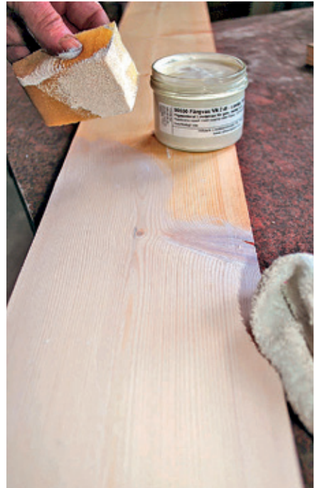
Apply the wax on untreated absorbent surfaces. Wipe with a dry cloth within about 20 minutes.
